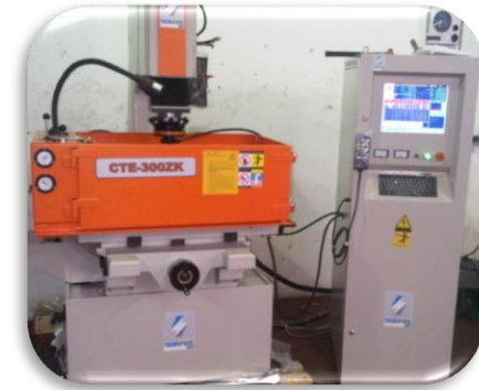
EROSION DE PENETRACION RECORRIDO 300mm x 200mm 50 A
